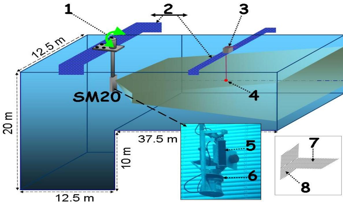
FIG. 1. (Color Online) Diagram of the instrumented seawater tank configured for multibeam sonar (MBS) calibration. 1) Automatic rotator (360° arc, 0.03° accuracy, PC control). 2) Moveable platforms. 3) Manual system with a ruler gauge for the vertical displacement of the sphere. 4) Tungsten-carbide calibration sphere or hydrophone. 5) MBS external transducer. 6) MBS sonar head. 7) MBS equatorial plane. 8) MBS polar plane.
