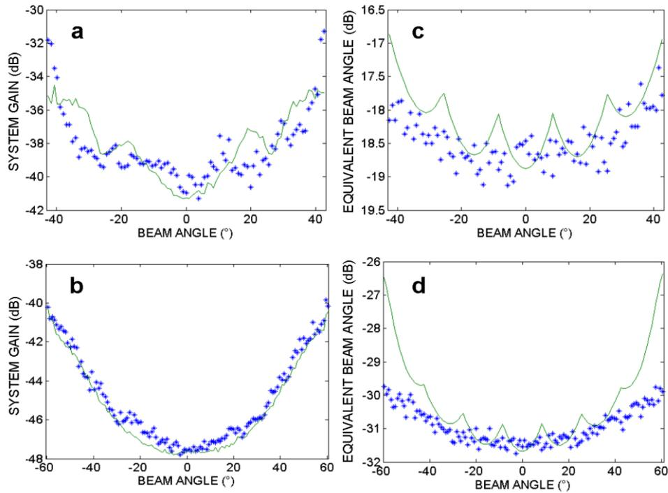
FIG. 6. Measured (\*) and estimated (solid) system gains (a) and equivalent two-way beam angles (c) for beam angles below  $\pm 40^\circ$  in IM imaging mode. (b-d) the same for all the beams in ES echo sounder mode.
