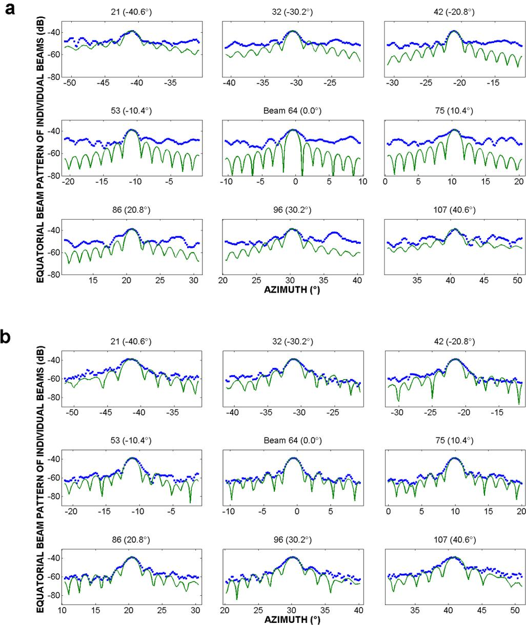
**FIG. 5. (a) Equatorial-plane two-way beam patterns, from the calibration sphere (\*) and estimated (solid), of a set of individual beams in IM imaging mode. (b) Equatorial-plane two-way beam patterns, measured from the calibration sphere (\*) and estimated (solid), of a set of individual beams of the SM20 multibeam sonar in ES Echo sounder mode. Text in each subplot indicates the beam number and its beam angle.**
