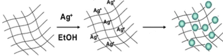
Fig 6 - Example of silver impregnation (figure adapted from [29]).
