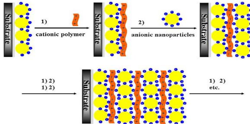
Fig 7- Layer-by-layer technique (figure adapted from [32]).
