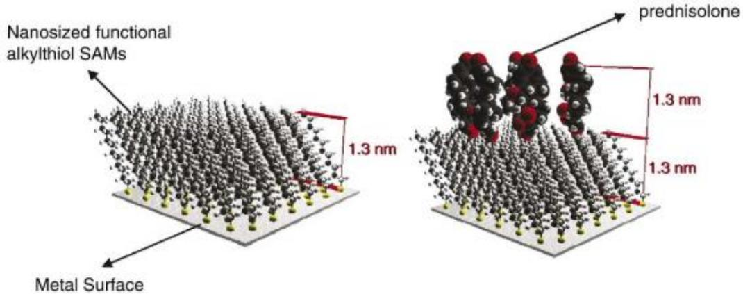
Fig 8- Representation of nanosized functional SAMs used as tethers for drug attachment and delivery for cardiovascular stents (image adapted from [34]).
