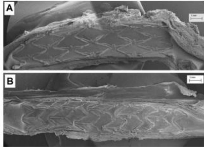
**Fig 10- SEM images (x35) after 7 days of stent coated (A) and uncoated stent (B) implantation (image adapted from: [40]).**
