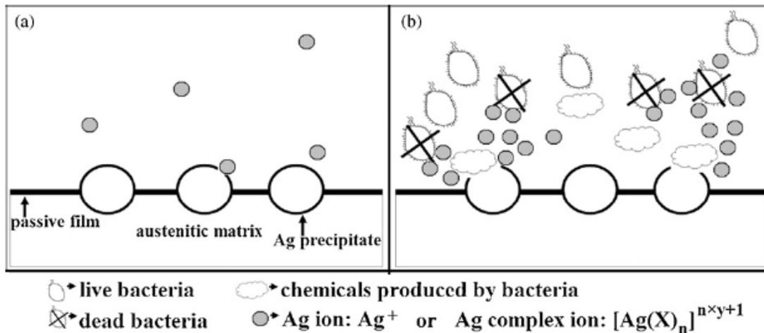
Fig 5- Silver antibacterial mechanism (image adapted from [26]).
