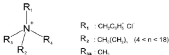
Fig 4- Quaternary ammonium compounds only have antimicrobial activity if the alkyl chain (R2) contains between 4 and 18 carbon atoms (figure adapted from [9]).
