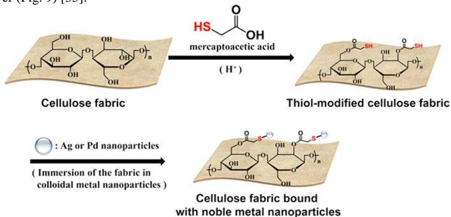
Fig 9- Example of covalent attachment (figure adapted from: [28]).
