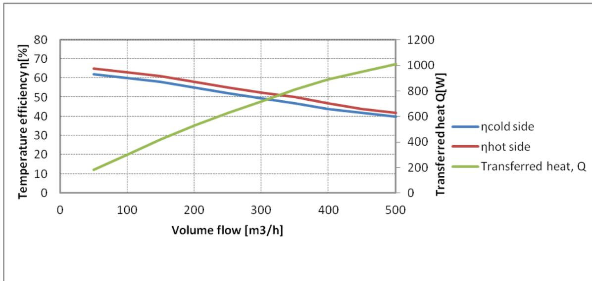
Fig 4. Graph against temperature efficiency vs volume flow (<http://www.segerfrojd.com/performance.htm>)
