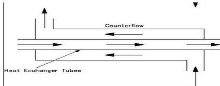
Fig 1. Counter flowing fluid in heat exchanger
