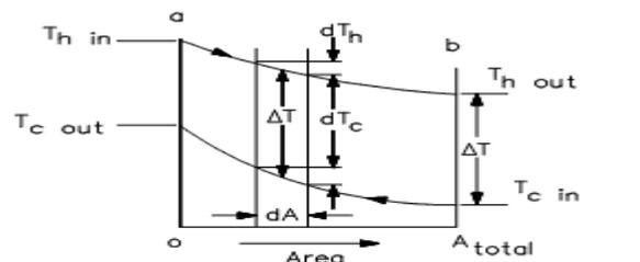
Temperature Distribution In Counter-Flow Heat Exchanger
