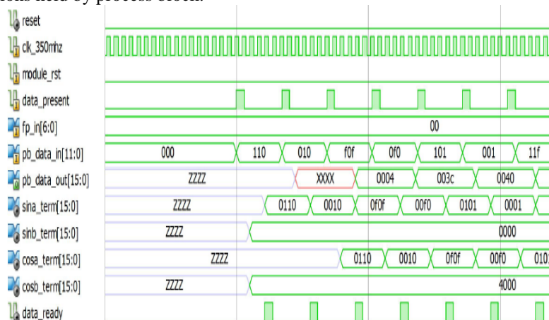
Fig 5: Complex multiplier output of a process block
