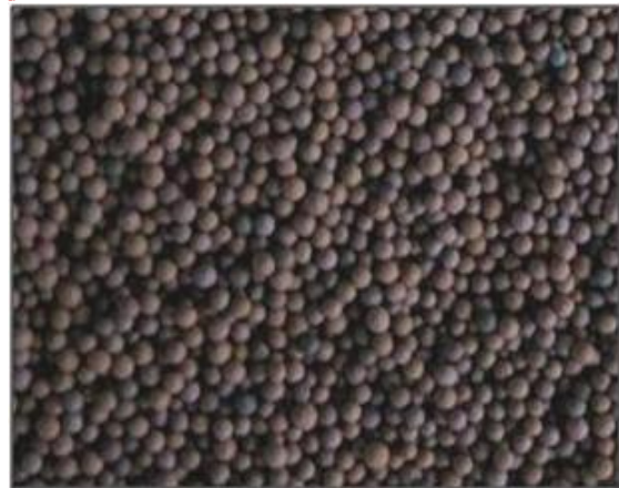
Fig. 4 BIOLITE media used in BIOFOR
