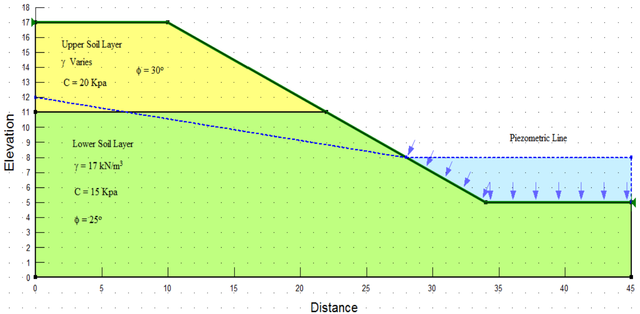
Fig 9 Profile and material property information for two-dimensional slope stability problem For different unit weight values
