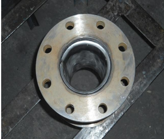
Fig 5: Actual photograph of bellows with liner
