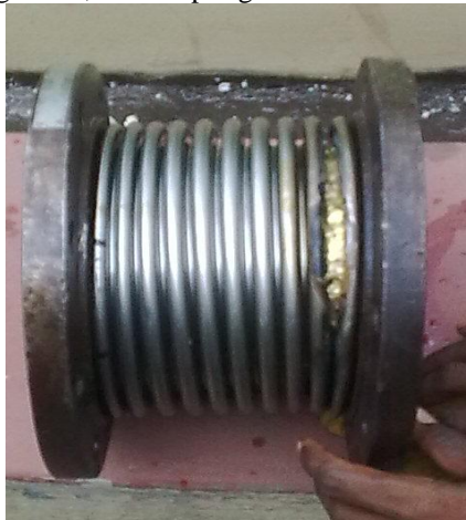
Fig 1: Sample photograph of fail bellows
