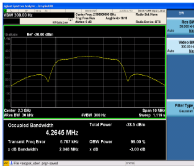
Fig. 6: Practical PCM/FM spectrum at 4 Mbps in S-band.
