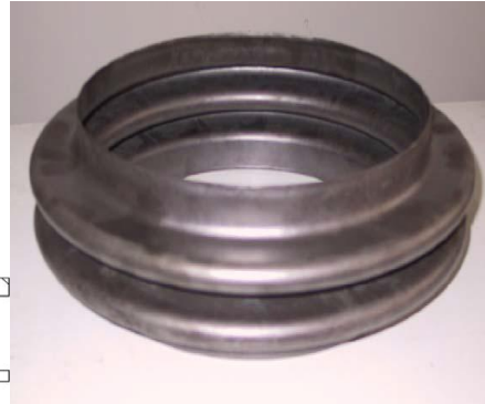
Fig-4 Photograph of the formed bellows of Ti-6Al-4V alloy
