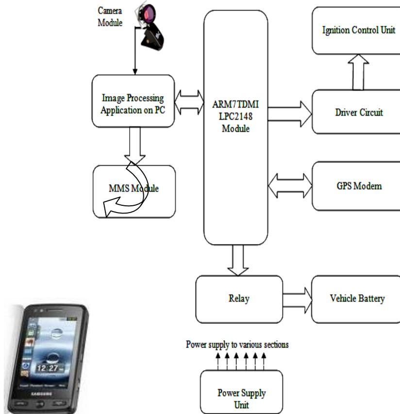
Fig 1. Block Diagram of Automotive Security System
